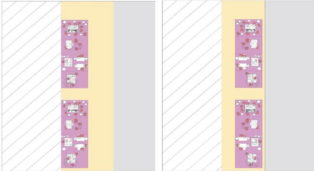
Figure 8 Optimal vendor placement within vending spaces: Facing carriageway for wider spaces (Left) and Facing Away from Carriageway for Limited Space (Right).
